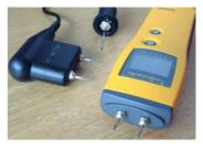
When used with the optional temperature probe (illustrated centre), the moisture measurements are automatically corrected with respect to temperature. This last feature is particularly relevant for users measuring wood that it significantly above or below 20°C.
